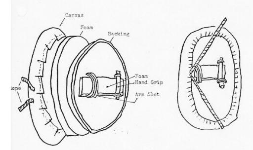
All shields must be covered with a layer of foam that is at 2" thick. The heavier the shield is the thicker the foam should be. Cover the foam with canvas. The height of your shield should not exceed the distance from your ankles to your shoulders. No circular shield can have a diameter over three feet. Any shield that is not a circle cannot be wider than 2 feet. All shields must either have foam folded over the edges, or have the shield recessed into the foam.
